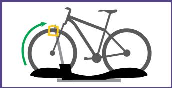
**3.** Raise support arm over front tyre so the hook rests on the front wheel. The bike is now secure and you can board the bus.
