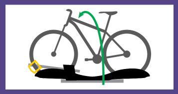
**2.** Lift bike onto rack with front wheel facing towards the yellow support arm.
